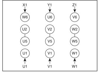
**Figure 6.** Model G0549 motor wiring for 440V operation.
